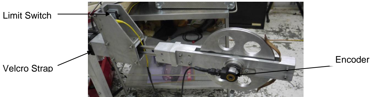
Figure 14 – Mast Cable Connections
