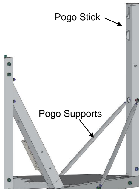
Figure 6 – Pogo Stick Installation
