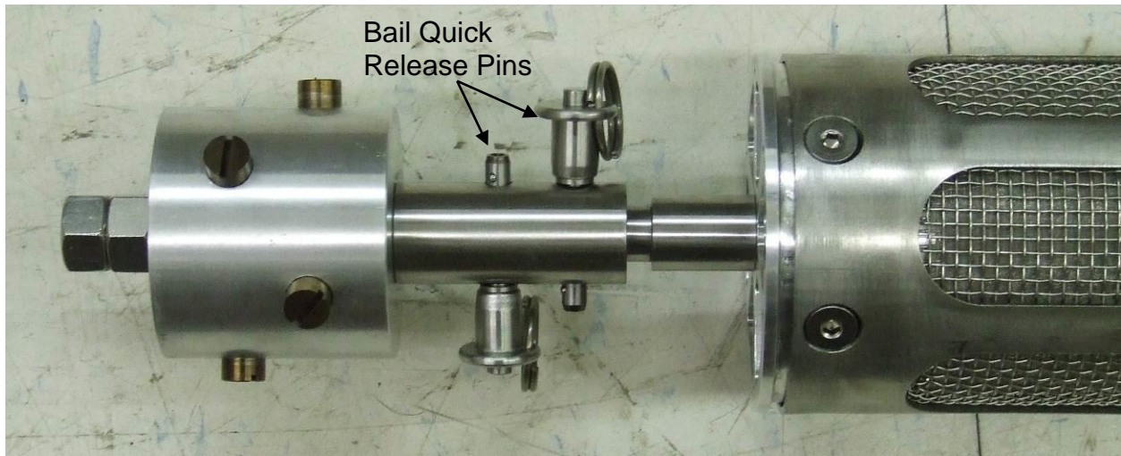
Figure 47 – Booster Pump Connection
